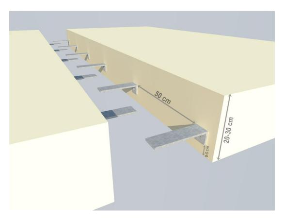
2. Screw the stainless steel holders to the side of the concrete. Make sure that holders are installed every 50 cm on each side. Holders should be cross-fixed assuring the support for Insulation Ropes practically every 25 cm.
