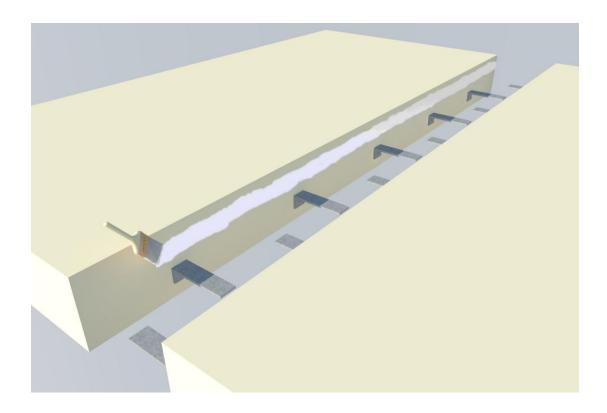
4. Take the Insulation Ropes, insert them into dilatation element and make sure they completely fit the part, where adhesive is applied.
